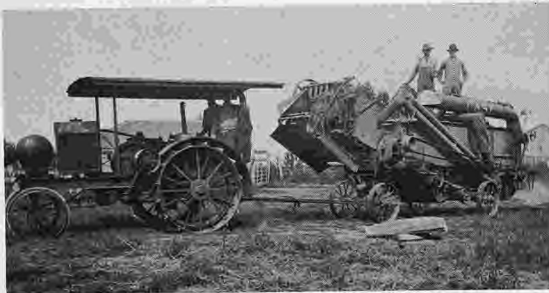
Early oil burning plow tractor, 1916 model, also used for threshing. Zeke and Virgil Goff on tractor; George and Gordon on separator.
